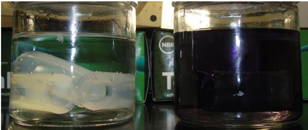
**Image 3:** Silicone Tubing (on left) and EPDM Tubing (on right) in IPA – day one (initial).
