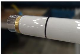
**FEP/PFA Coating** can be directly applied onto a substrate like light bulbs, steel pipes, and cables. A homogeneous thin film of fluoropolymer is directly extruded onto the substrate by a continuous process and avoids an additional shrinking step in the process. The fluoropolymer coating provides shatter protection for the light bulbs, shields pipes and cables from corrosion and weathering while providing transparency and anti-stick properties.
