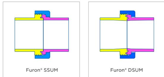
After 48 hours of continuous testing, the components were removed from the vibration unit and subjected to the bubble test again. No bubbles appear during the one minute test period for either the SSUM or DSUM fitting design.
