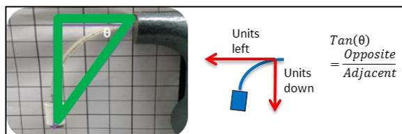
**Figure 1. Left – deflection test configuration showing clamped sample (fuel line and filter) and background grid. Right – calculation of the deflection angle as a measure of sample flexibility.**
