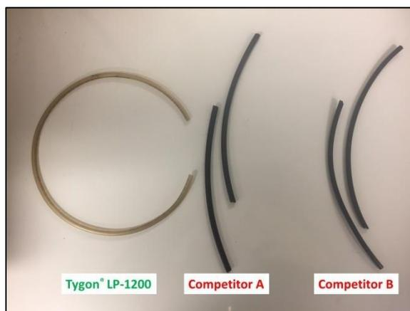
**Figure 5. Test samples after low temperature bend testing. Competitors A and B both snapped in half. Tygon® LP-1200 passed the test.**
