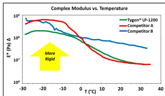
Figure 4. DMA testing on fuel tubing samples. Complex modulus of LP-1200 and Competitor A as a function of temperature. Modulus of Competitor A increases dramatically as temperature is lowered.
