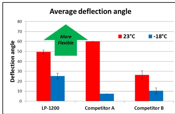
Figure 2. Deflection angle at room and low temperatures for Tygon® LP-1200 vs Competitors A and B. Higher deflection angle indicates higher flexibility.
