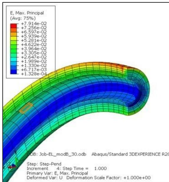
Figure 3. Strain fringe plot of two-layer tube (cross-sectioned) at a 30-degree orientation of gravity loading.
