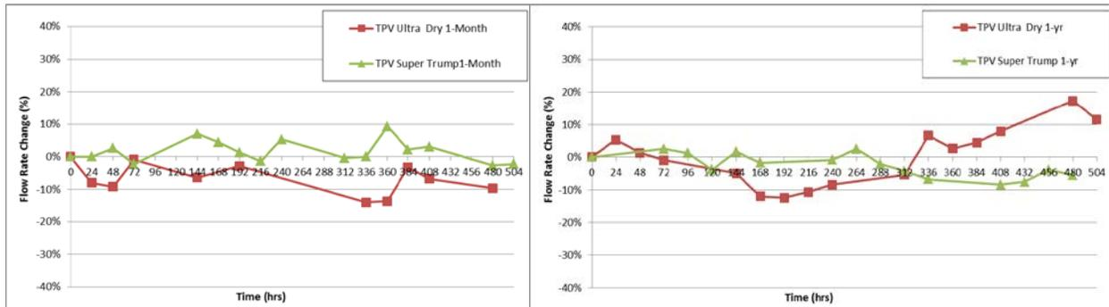
Figure 7: Effect of chemical exposure and time on thermoplastic vulcanizate (TPV) tubing performance
