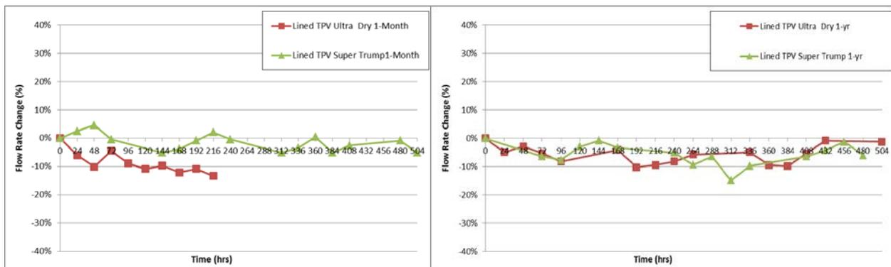
Figure 8: Effect of chemical exposure and time on lined thermoplastic vulcanizate (lined TPV) tubing performance
