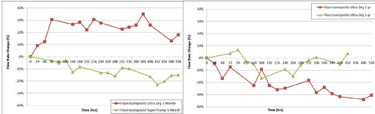
Figure 5: Effect of chemical exposure and time on composite fluoroelastomer tubing performance
