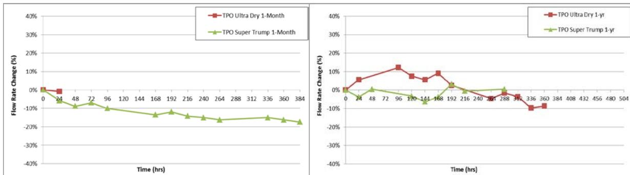
Figure 6: Effect of chemical exposure and time on polyolefin elastomer (TPO) tubing performance
