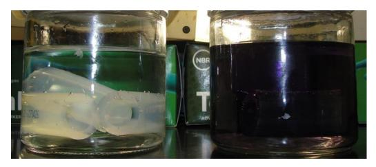
Image 3: Silicone Tubing (on left) and EPDM Tubing (on right) in IPA – day one (initial).
