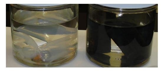
**Image 4:** Silicone Tubing (on left) and EPDM Tubing (on right) in IPA – 72 hours.
