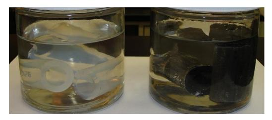
**Image 2:** Silicone Tubing (on left) and EPDM Tubing (on right) in 0.5% nitric acid – 72 hours.
